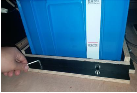
Step 1: Remove the screws of tank baffle.
