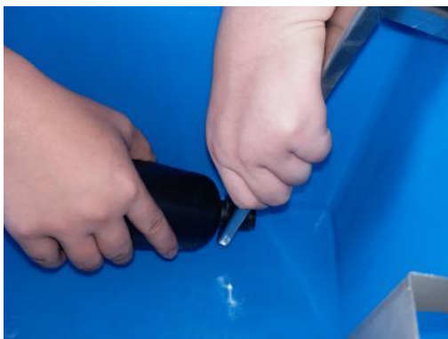
Step 5: Remove the secondary filter as shown in the following two figures.
