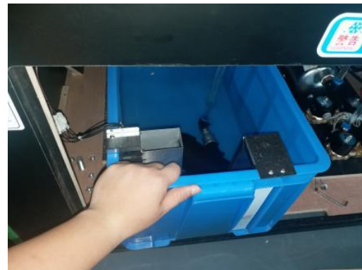
Step 4: Gently pull out tank by 1/3.connector.
