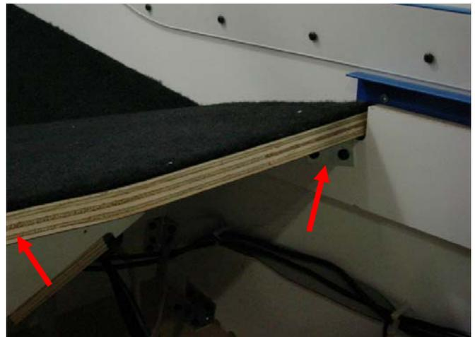
Remove screws from brackets holding vertical wood that sensor is mounted to.
