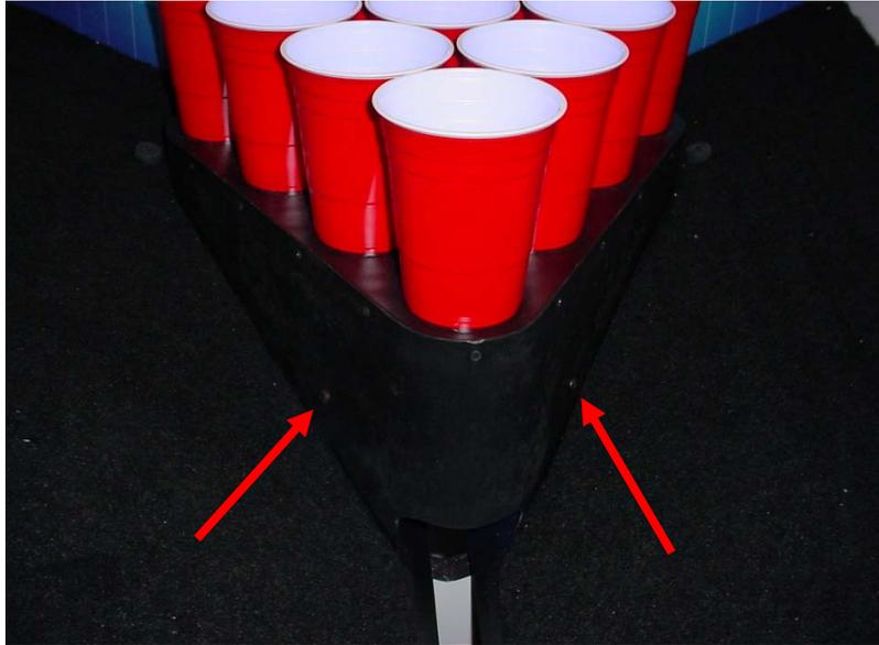
Remove 2 screws holding cup platform in place.
