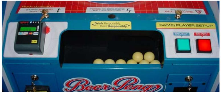
The E-Port Reader will involve drilling holes in the left side of your metal front to mount. Instructions will come with E-Port Reader, here is a picture of it mounted on metal plate.
