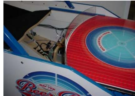
Remove 2 screws from brackets on both sides of the cabinet and remove carpeted wood platform.
