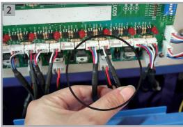
■Once the wire unpluged, the Frog Head is able to removed and put the new Frog Head instead.
