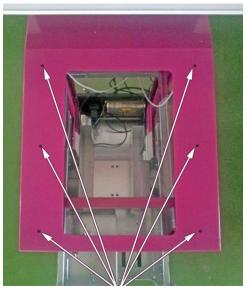
Place the threads in the lower part of the panel in the holes located on the oblique part of the device and attach it on the inside, with accompanying nuts.
