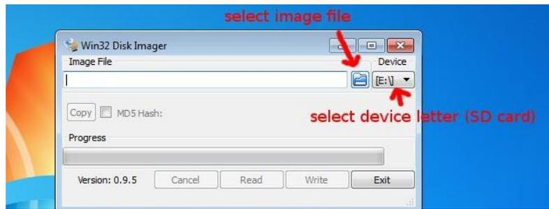
6. When image file and drive letter is selected properly, click “Write” and wait for finish. Put SD card back into CPU board unit and turn the machine on. Solid RED and blinking BLUE LED light on CPU board means that everything is ok. (refer to other “Troubleshooting” steps)
