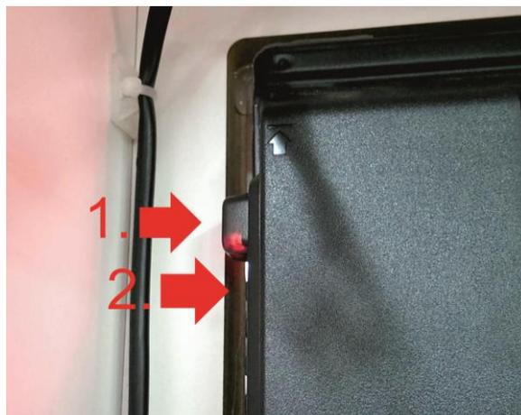
3. Check CPU board (1st step of „No signal alert on screen”)
