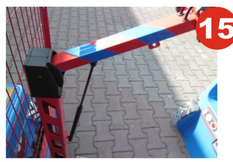
Place the spreader between the vertical and the middle arm
