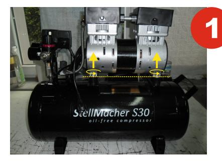
Remove the engine from the compressor cylinder. Signal cable between cylinder and the engine may require extension
