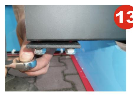
Screw vertical arm to the base. Remember to use pads under the screws
